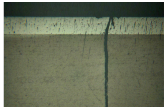
50X section view of 12 mil chrome layer (.012") showing crack propagating into ram base metal
