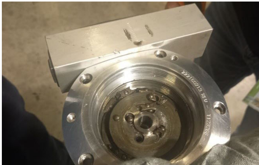
Figure 1-1. Necker Reform Head Failure
