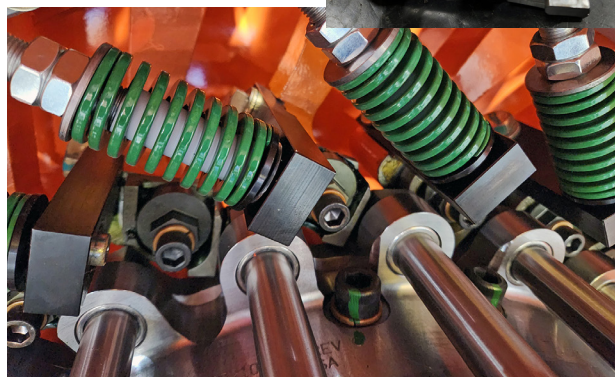
New wear plate design allows replacement of a wear part instead of the entire rest shaft bracket
