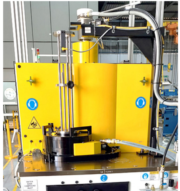
Existing 1 piece guard on a VHSL Liner
