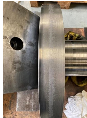
Above and Left: Photos showing excessive wear in bearings caused by improperly filtered lube oil
