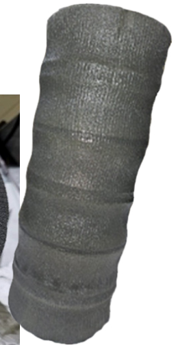
Below: Low quality non-OEM filter canister and media
