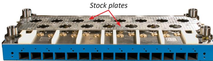
Previously, the custom shaped stock plate bolts were machined from bar stock. The external threads of the bolt engaged with internal threads machined into the piston. Customers have alerted us to situations where they were not able to remove the stock plate bolts from the pistons with a conventional hex wrench because the threads may have corroded, galled or fractured due to various reasons.
