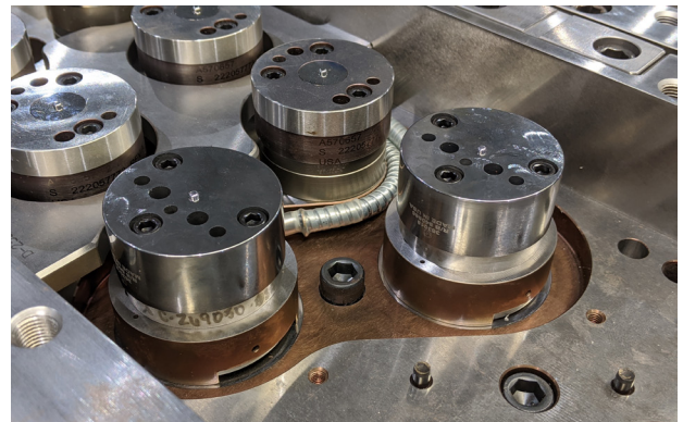
Thermal score anvils installed in a lane die of a Tetrad beer-beverage EOE conversion system
