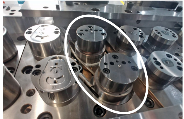
Thermal score anvils installed in a lane die of a Tetrads beer-beverage EOE conversion system
