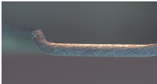
*Second operation tooling (left) performs the hem wipe-up (above) on the edge of the rivet hole*
