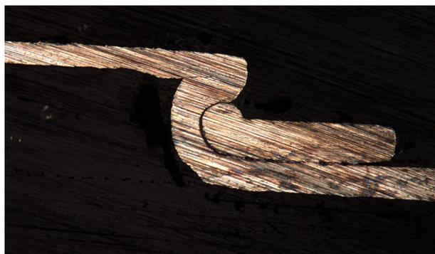
*Stake station tooling (above) and close up of hemmed rivet hole and rivet after the stake operation (below)*
