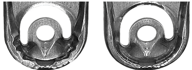
Tab with standard nose curl (left) and X1 technology curl (right) showing how wrinkling is controlled. This photo also clearly shows the "long leg - short leg" tongue shape.
