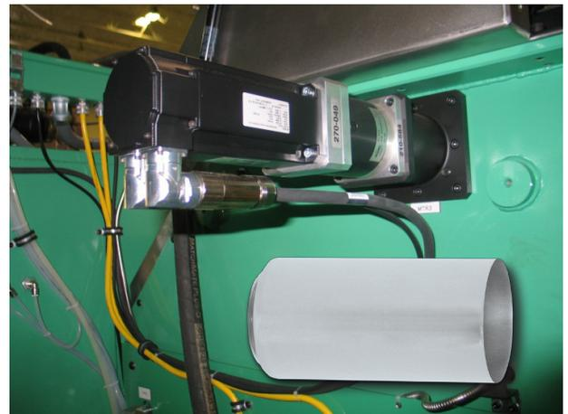
Ragsdale can unloader servo motor and gearbox
