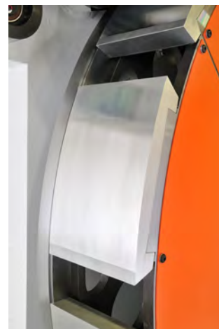
Replaceable aluminum segments on cantilevered blanket wheel
