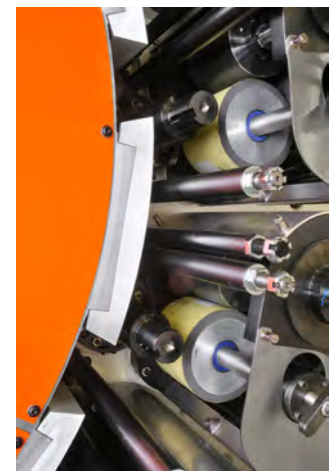
Full running registration features on plate cylinder shaft assemblies
