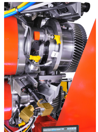
Concord plate cylinder showing the 3 adjustments accomplished by the Remote Registration system
