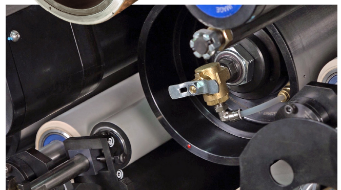
Air valve on the end of the plate cylinder shaft that is turned on when changing the plate sleeve
