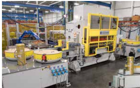
FLEXOR sheet feed shell and end system features a lower cost portal press and a robotic sheet feed system
