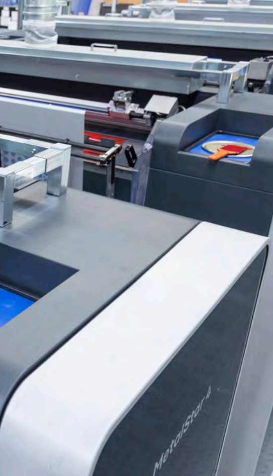
Belvac’s decorator, with a printing sleeve that enables higher-definition printing
