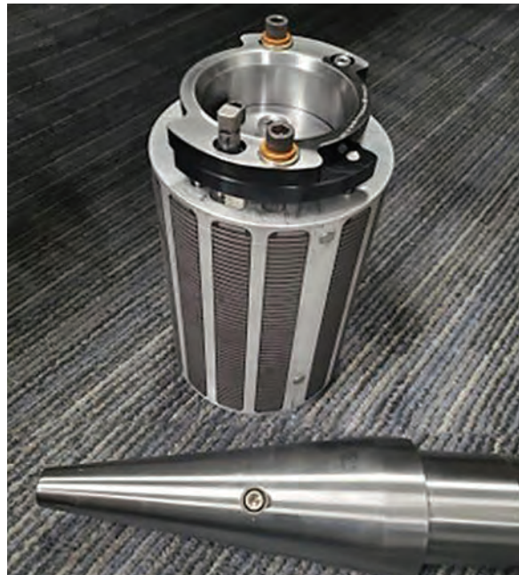
Above Installed as standard on Rutherford Decorators, the tapered shaft plate cylinder is designed to enable a precise fit
