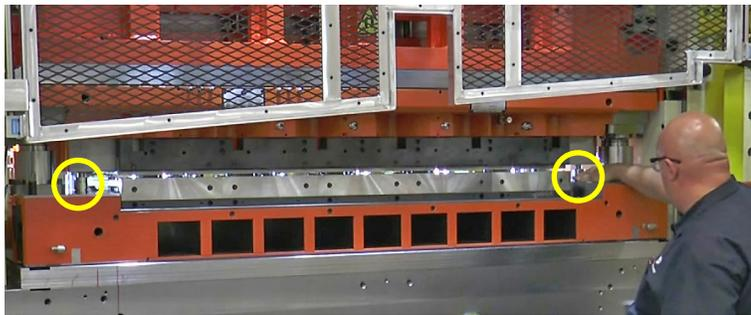
*Installing the gas cylinder installation fixtures in a cupping die set*
