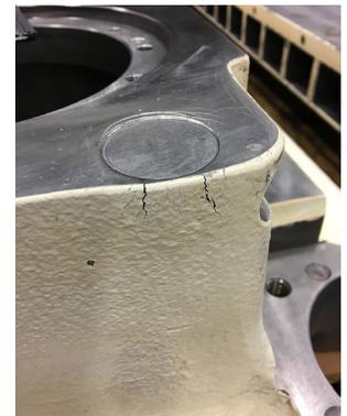
*Cupping die shoe damage caused by lowering the upper press slides with traditional solid parallel blocks in place*
