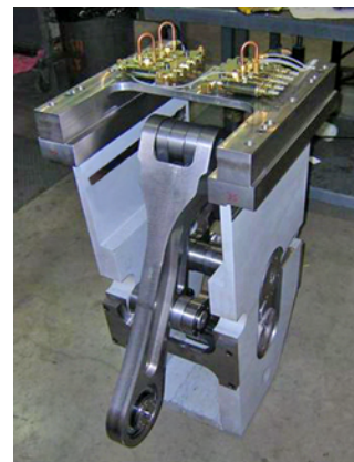
Integrated lubrication system connections at top of modular assembly
