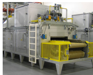
Above: Specially-designed Inside Spray Machine is available with servo-controlled lance or fixed gun
